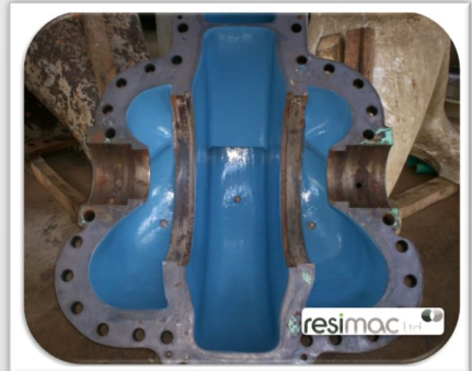
Split Case Pump Volute Repaired and Protected with Resimac 203 SuperFlow
