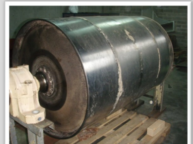
Resimac 202 Ceramic Fluid adds Anti-Slip to this Drive Pulley
