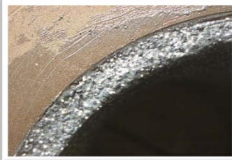
Damaged Spool Rebuilt with Resimac 204 Heavy Duty Paste and Protected with Resimac 202 Ceramic Repair Fluid
