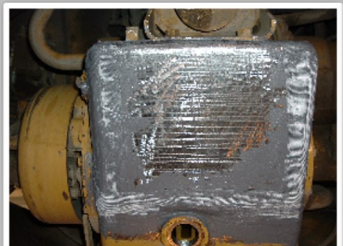
Cold Weld Plate bonded Repair with Resimac 101 Metal Repair Paste
