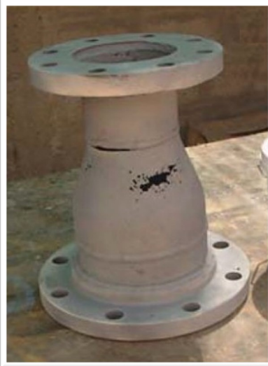
Damaged Spool Rebuilt with Resimac 204 Heavy Duty Paste and Protected with Resimac 202 Ceramic Repair Fluid
