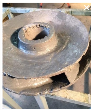
Oily Metal Flange Sealed with Resimac 104 Metal Repair Fluid
