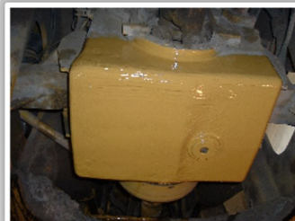
Cold Weld Plate bonded Repair with Resimac 101 Metal Repair Paste
