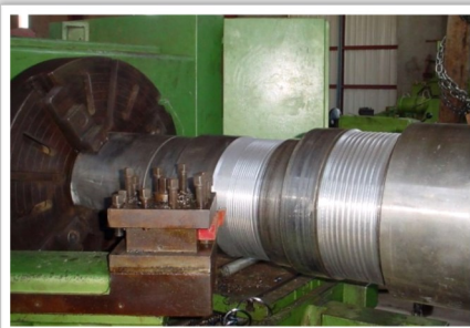
Worn Shaft Surface Rebuilt with Resimac 101 Metal Repair Paste and then Machined on a Lathe
