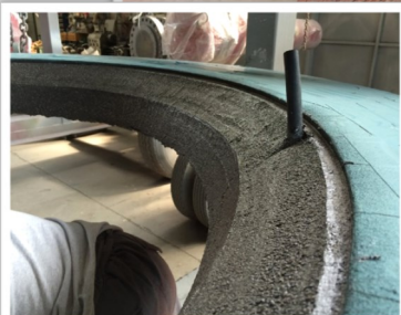
Damaged Turbine Cover Rebuilt with Resimac 204 Heavy Duty and Protected with Resimac 202 Ceramic Repair Fluid
