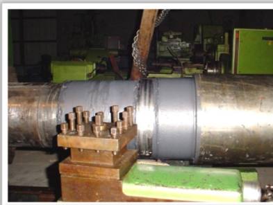
Worn Shaft Surface Rebuilt with Resimac 101 Metal Repair Paste and then Machined on a Lathe
