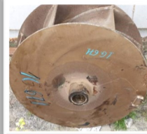
Split Case Pump Volute Repaired and Protected with Resimac 203 SuperFlow
