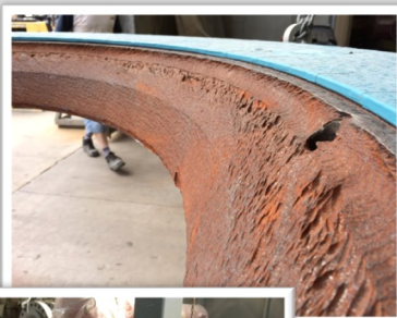
Worn Shaft Surface Rebuilt with Resimac 101 Metal Repair Paste and then Machined on a Lathe
