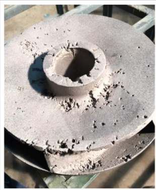
Oily Metal Flange Sealed with Resimac 104 Metal Repair Fluid
