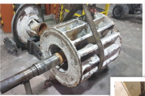
Several Pump Components Rebuilt and Protected with Resimac materials
