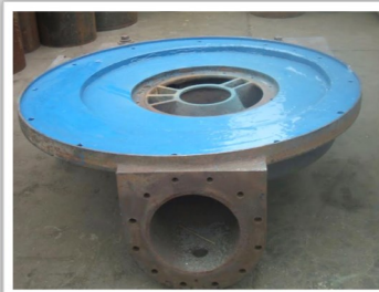
Several Pump Components Rebuilt and Protected with Resimac materials
