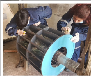
Cold Weld Plate bonded Repair with Resimac 101 Metal Repair Paste
